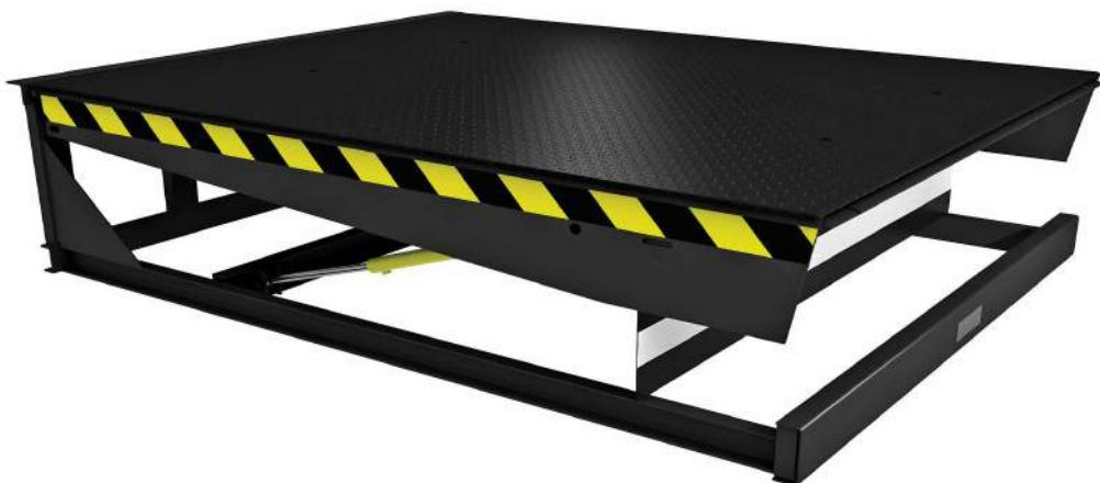
DSI electrohydraulic dock leveler with telescopic lip is the most efficient device, which enables access of a forklift from the warehouse to the truck bed when loading/unloading. It is used, when there is a need in exact positioning of the lip on the truck bed, for instance, if the truck is not correctly parked, or if side loading is to be performed. Lip segments allow to load/unload the trucks, which is less than width of the dock leveler.
