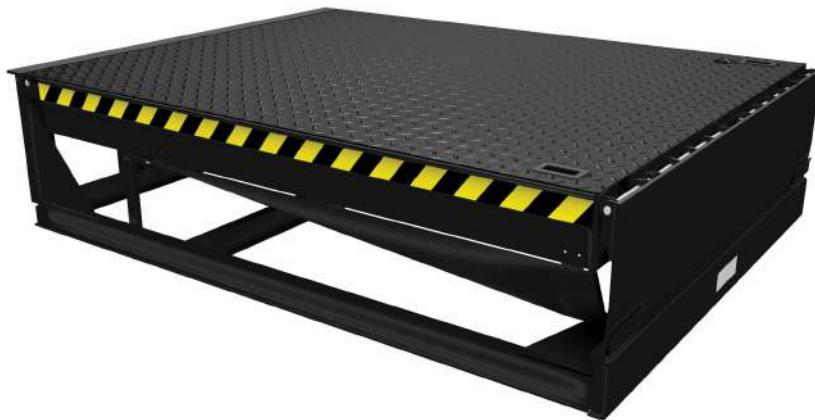
MODL mechanical dock leveler does not require power supply and is a good alternative to the electrohydraulic dock leveler in case power supply is not available. Manual efforts of 2 people are needed to rise the upper deck, at that the lip turns and opens automatically. Then the deck lowers until it rests on the truck bed. After loading/unloading is completed, the lip lowers; the deck rises and returns to its rest position. Dock leveler can be installed by either embedded or suspended way.
