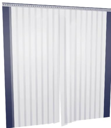
DoorHan strip PVC door of FS series is a set of transparent film strips which are hanged using a fastening. It is easy-to-mount and easy-to-clean. Standard or low temperature film is used, which allows operation of this door at low or high temperatures. The material has high tear resistance and tensile strength, good sound insulation, UV-radiation protection and flexibility. All strips have rounded edges to ensure safety and durability.
