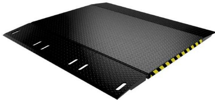
MT mobile tracks are used for loading/unloading when standard dock leveler or folding track can not be used. They are designed for using with trucks which have approximately the same height above the ramp level. The mobile track can compensate height difference up to 240 mm. The track can be transported to the required place using a forklift. Mobile tracks of MT series comply with rules and regulations of the European Standard EN 1398.
